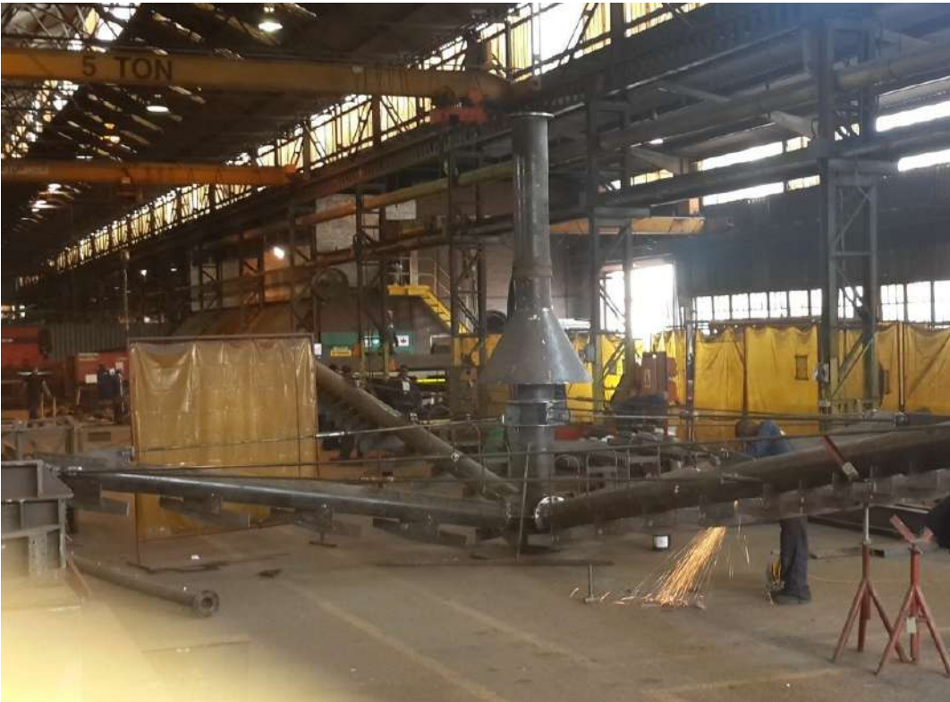
Trial fit-up of rake arms to torque tube
