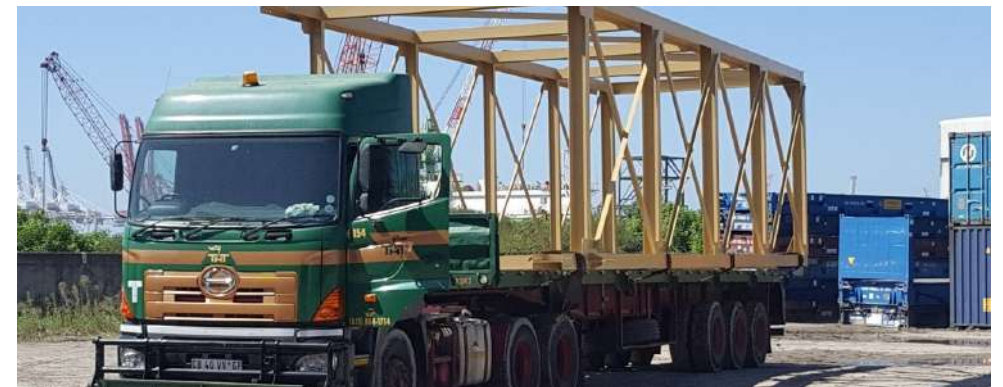
12 m bridge fully assembled
