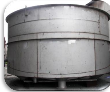
Stainless Steel Drop Separator for Boiler
